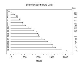
Failure Pattern in the Bearing Cage Data
